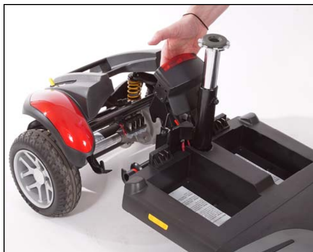
Figure 17. Separating the Drivetrain and Frame
