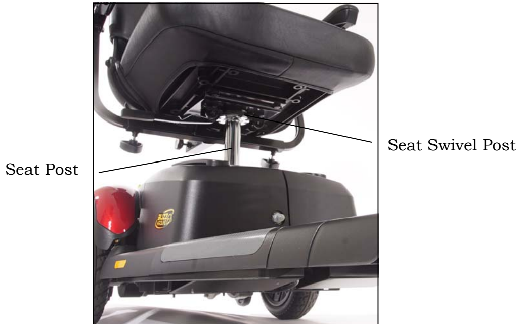
Figure 23. Installing the Seat
