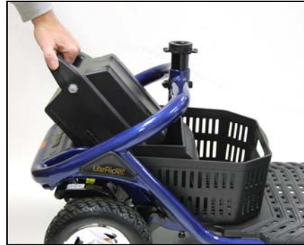
Figure 21. Battery Pack Installation
