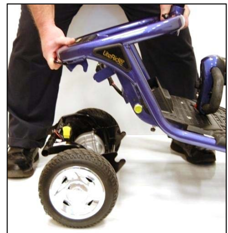
Figure 18. Lifting the Frame
