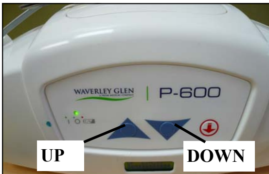
Figure 5C - Front Panel showing raising/lowering buttons
