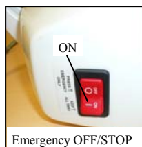
Figure 14D - Close-up of switch ON - Normal lift Operation OFF - Emergency Stop
