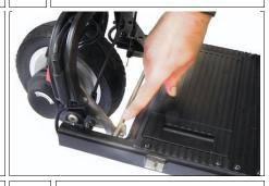
\_the scooter will unfold as you pull the seat back and steering column apart and \_
