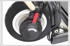
...if not press your foot down onto the footplate to lock the scooter open. If not already installed apply the seat cushions and seat back as shown.
