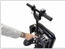
To turn the scooter into rolling luggage ensure the vertical steering column is locked against the steering column latch.
