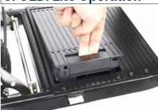
The battery can be removed by lifting the latch and lifting upwards.
