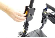
Press and hold the small yellow latch on the steering column...
