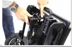
and steering column latch locks into positiion.
